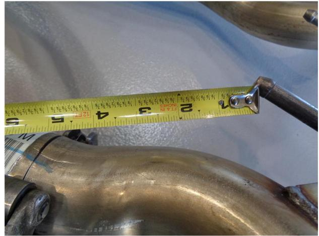
**Step 2.** Begin removing the OEM exhaust system by cutting both pipes exiting the resonator. Measure and cut on the driver side 5" from the tip of the hanger. Cut the passenger side also from the tip of the hanger 5.5" back. Next, extract the hangers from the rubber insulators and remove the OEM mufflers. Retain insulators as they will be used to install the new system.
