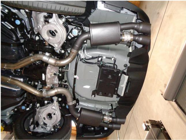
**Step 4.** Next attach both Muffler Assemblies to the Inlet Pipe Assemblies using the supplied 3.00" clamps and fitting the hangers into the rubber insulators.
