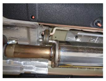
**Step 2.** Begin installation of your new MAGNAFLOW system by slipping the Resonator Assembly inlet end over the Catalytic Converter outlet. Loosely secure using the supplied 2.36" clamp. Leave all clamps loose during initial installation.
