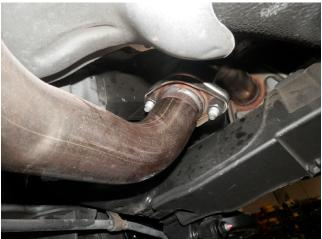
**Step 1.** To remove the OE exhaust you will need to cut the exhaust pipe 3.00" rearward of the catalytic converter as shown (remove heatshield first). Deburr the cut edges. Unbolt the flange junction beween the OE mid pipe and muffler assembly. Disengage all welded hangers from the rubber insulators. Retain rubber insulators as they will be needed to install your new MAGNAFLOW system. The OEM system can now be removed.
