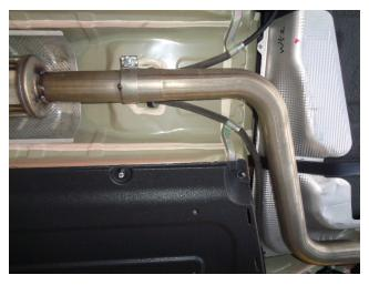
**Step 3.** Next, install the Mid-Pipe Assembly using the supplied 2.50" clamp.
