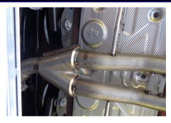
Step 4. Complete the assembly by attaching the Tailpipe Assembly to the Mid-Pipe Assembly using the supplied 2.50 clamp and engaging the hangers into the rubber insulators.
