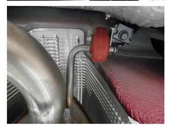
**Step 1.** Begin removal of the OEM system by loosening the clamp at the inlet of the Resonator and removing the black tubular cross brace, you can then disengage the welded hangers from the rubber insulators. Working rearward finish removing the system. Do not damage or discard the rubber insulators or OEM clamp as they will be re-used to mount the new system.
