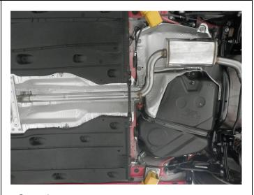
**Step 2.** Begin installation of the new system by attaching the Inlet Pipe to the factory outlet using the OEM clamp and fit the hanger into the rubber insulator. Leave all clamps loose until final adjustment. Next Install the Muffler Assembly using the supplied 2.50" clamp and fit the welded hanger on the assembly to the previously un-used hanger on the underside of the vehicle using the supplied rubber insulator.
