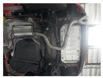
**Step 3.** Next Install the Tailpipe Assembly using the supplied 2.50" clamp and fit the welded hanger into the rubber insulator. Re-attach the tubular cross brace.
