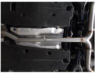
Step 2. Begin installation of the MagnaFlow system by attaching the Resonator Assembly to the outlet of the catalytic converter using the OE fasteners. Next, attach the Extension Pipe and Y-Pipe Assembly using the supplied 2.50" clamp and engaging the hanger into the rubber insulators. (Leave all clamp and fasteners loose for final adjustment of the complete system.)
