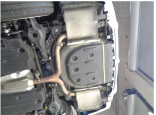
Step 1. To remove the OE exhaust system begin by unfastening the 2 bolt flanges, one located at the front of the vehicle (behind the catalytic converter assy) and one at the rear (by the muffler). Working front to rear disengage the hangers from the rubber insulators and remove the exhaust. Do not damage the rubber insulators and retain the front flange hardware as they will be used to install the new exhaust system.
