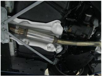
**Step 3.** Loosely install the Inlet Resonator Assembly using the supplied 3.25" clamp.
