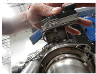
**Step 4.** At this point the OEM exhaust control valve motor can be bolted to the valve assembly on the new Muffler Assembly. Align the keyways in the valve motor and shaft of the new valve. Mate both keyway notches using the OEM indexing spring. Secure the valve motor using the three supplied mounting bolts. \*\*NOTE: Do NOT loosen or undo the V-Band Clamps, they are designed for one time use only. Once the clamp is tightened it can not be reused.
