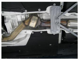
**Step 2.** You will need to cut the OEM exhaust pipe at the inlet weld of the stock resonator. Disengage all welded hangers from the OEM rubber insulators. Do not discard the OEM fasteners or damge the rubber insulators as the will be needed to mount your new MAGNAFLOW system. Once the OEM system has been removed you can unbolt the exhaust control valve motor. Be sure to retain the indexing spring shown in the diagram for Step 1.
