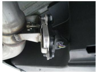
**Step 1.** To remove the OEM exhaust system you will first need to unplug the exhaust valve control motor located on the OEM muffler assembly.
