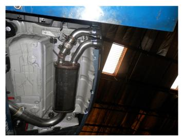
**Step 5.** Loosely attach the Muffler Assembly to the Inlet Assembly using the supplied clamp. Engage all welded hangers to the rubber insulators.
