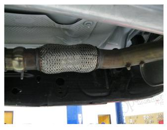
**Step 1.** To Remove the OEM system, you will need to cut the exhaust pipe behind the muffler before it goes over the axle. Next disengage the welded hangers from the rubber insulators and remove the tail pipe. Unclamp the muffler inlet from the catalytic converter at the clamp junction. Do not damage or discard the OEM fasteners or rubber isolators, as they will be reused to mount your new MAGNAFLOW system.
