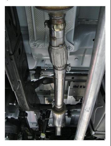
**Step 2.** Install the new Inlet Pipe Assembly at the ball flare using the OEM fastener. Install the Mid Pipe Assembly by slipping the inlet over the outlet of the Inlet Pipe Assembly. Then loosely secure using the supplied 3.00" clamp.
