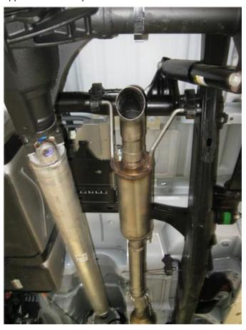
**Step 3.** Install the Mufflerr Assembly and tail pipe following the same procedure using the supplied 2.50" clamps and by fitting the welded hangers into the OEM rubber isolators. Leave all clamps and fasteners loose for final adjustment of the complete system.
