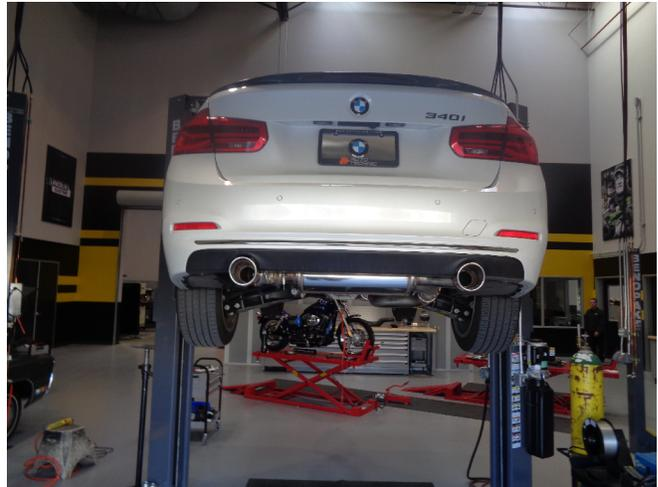
Step 6: Once a final position has been chosen for the new exhaust system, evenly tighten all clamps from front to rear using the torque specifications on page one of these instructions. Inspect all fasteners after 25-50 miles for operation and re-tighten if necessary.
