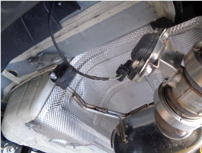
Step 2: Before installing your new system attach the OE valve motor to the valve on the Magnaflow Muffler Assembly using the OE hardware.
