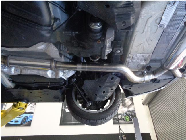
Step 4: Loosely attach the Resonator Assembly Inlet to the Inlet Pipe Assembly outlet with the supplied clamp. Install the Extension Pipe to the Resonator Assembly the same way.
