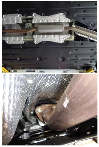
Step 1: To remove the OEM system first unbolt and remove the cross member at the inlet. Next, unbolt the inlet pipe at the catalytic converter flange junctions. Working front to rear disengage all welded hangers from the rubber insulators. The OEM exhaust system can now be removed in one piece. Be sure to retain all mounting hardware as it will be needed to install your new MAGNAFLOW system
