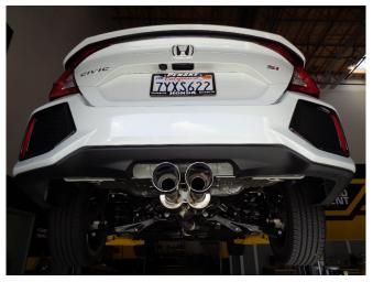
Step 5: Once a final position has been chosen for the new exhaust system, evenly tighten all clamps from front to rear using the torque specifications on page one of these instructions. Inspect all fasteners after 25-50 miles for operation and re-tighten if necessary.
