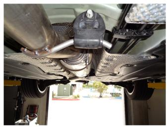
Step 2: Begin installing your new system by loosely bolting both inlet flange of the Inlet Assemblies to the catalytic converter outlets using the OEM hardware. Engage the welded hangers to the rubber insulator.
