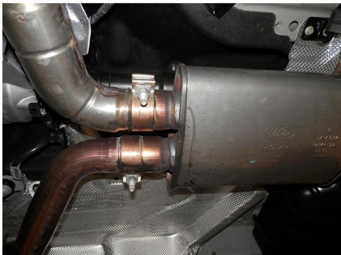
**Step 1.** Begin removal of the OEM system by unclamping the OEM muffer from the catalytic converter outlet pipes. You can then disengage the welded hangers from the rubber insulators, working rearward finish removing the system. Do not damage or discard the rubber insulators as they will be re-used to mount the new system.
