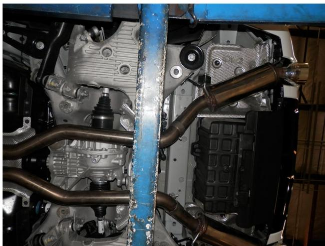
**Step 3.** Next loosely install the two Mid Pipe Assemblies and the muffer assemblies using the supplied 2.50" clamps. Engage the welded hangers to the rubber insulators.
