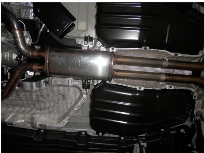
**Step 2.** Begin installation of your new MAGNAFLOW system by attaching the Inlet Muffer Assembly to the two catalytic converter outlet pipes. Loosely secure using the supplied 2.36" clamps. Fit the hangers into the rubber insulators. Leave all clamps loose until final adjustment.
