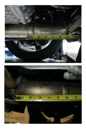
**Step 2.** You will need to cut the OEM exhaust system to remove it and install the new Magnaflow system. Measure and cut 6.00" forward of the hanger on the passenger side and driver side pipes. Remove mufflers and retain rubber hanger insulators to install the new system
