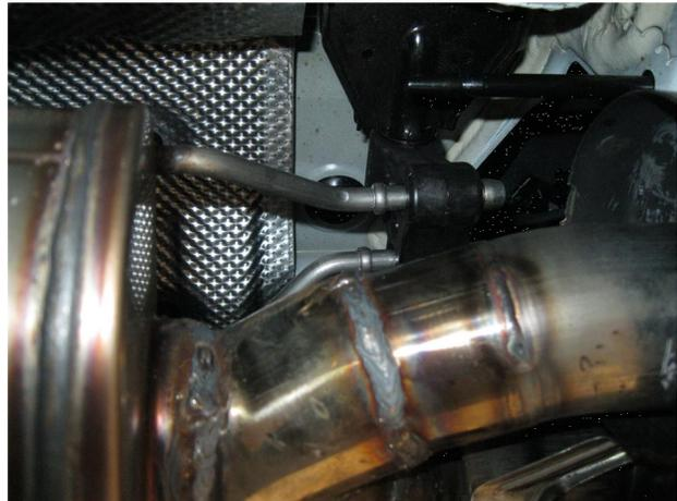
**Step 3.** Next Install the Mid-Pipe Assemblies to the outlets of the Resonator Assembly and then the Muffler Assemblies to the Mid-Pipes using the supplied 2.50" clamps. Insert hangers into rubber insulators. Re-attach brace.
