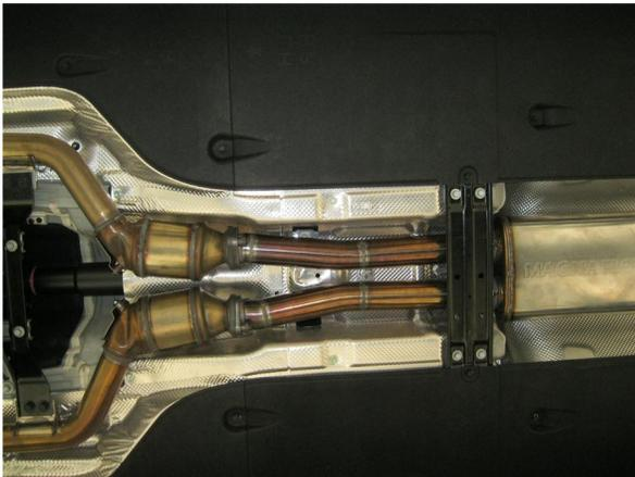
**Step 2.** Begin installation of the new system by fastening the Resonator Assembly inlets to the catalytic converter using the OEM fasteners and supplied gaskets (Leave all clamps and fasteners loose for final adjustment of the complete system.)
