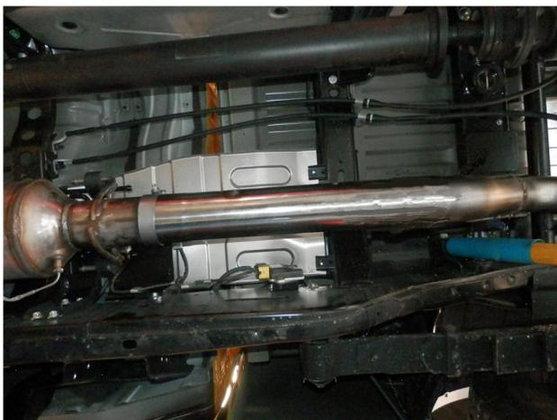
**Step 2.** Begin installation of the Magnaflow system by locating the indexing notch to the OEM peg then loosely clamping the Inlet Pipe to the outlet of the DPF using a supplied 4.00" clamp. Install the Over Axle Pipe in a similar fashion
