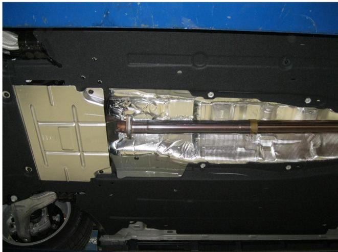
**Step 3.** Begin installing the new system by loosely bolting the flange of the Inlet Pipe Assembly for the outlet flange of the OEM catalytic converter using the supplied bolts and OEM hardware. Keep all fasteners and clamps loose until final adjustment.
