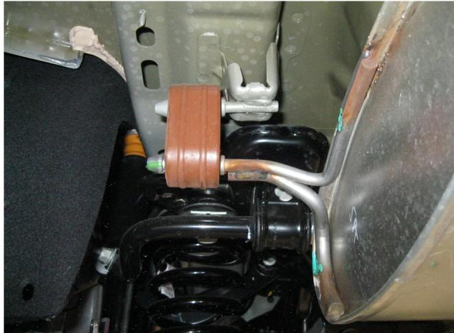
**Step 2.** Next, remove the welded hangers from the rubber insulators located on the OEM muffler and tail pipe assembly. The exhaust may now be removed in one piece.
