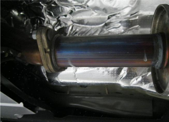
**Step 1.** To remove the OEM exhaust system you will first need to unbolt the OEM system inlet flange from the catalytic converter outlet pipe. Be sure to retain all mounting hardware as it will be needed to mount your new MAGNAFLOW system.
