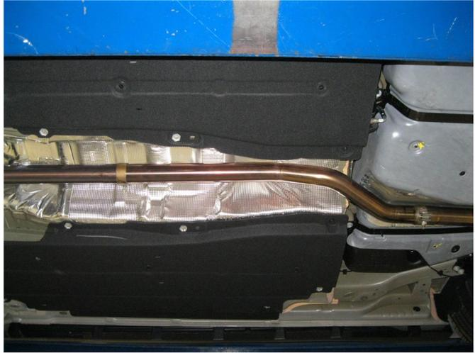
**Step 4.** Next slip the inlet of the Front Mid Pipe into the Inlet Pipe Assembly and loosely secure using the supplied 2.50" clamp.
