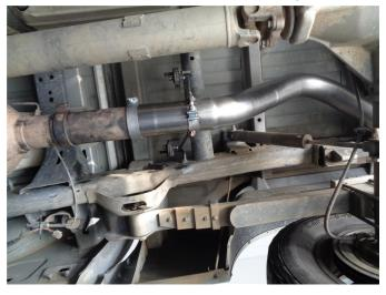
**Step 3.** Begin installation of the Magnaflow system by clamping the Inlet Pipe or Over Axle Pipe (depending on vehicle configuration) to the outlet of the DPF using a supplied 4.00" clamp. Locate the alignment notch to the OEM outlet. Slide the Hanger Clamp Assembly over the pipe and locate the welded hangers in the rubber insulators (leave all clamps loose for final adjustment of the complete system).
