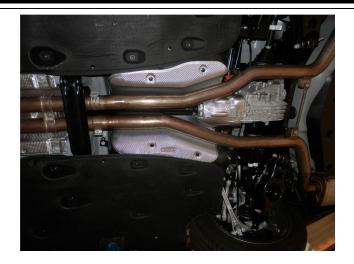
**Step 1.** Begin removal of the OEM exhaust system by loosening the two 3.00" clamps located behind the rear black cross brace.
