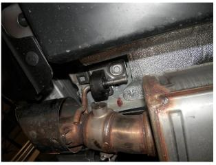
**Step 2.** Next, remove the tubular support brace connectiing the right and left exhaust, remove the right and left vacuum line from the exhaust valves (plug and zip tie out of the way, these will NOT be re-used), remove hangers from rubber insulators and drop the exhaust. Retain rubber insulators as they will be re-used on the new system.
