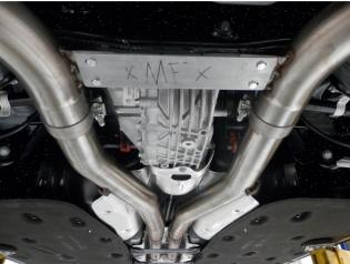
**Step 4.** Next, install the Driver and Passenger side muffler assemblies to the outlets of the Inlet assemblies using the supplied 3.00" clamps and fit the hangers into the rubber insualtors. Loosely Fit the Magnaflow cross brace using the supplied fasteners.
