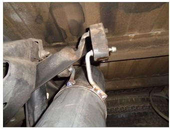
**Step 4.** Loosely install the Over Axle Pipe Assembly using the supplied clamps. Locate both hangers to the rubber insulators.
