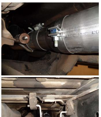
**Step 3.** As you assembly the Extension Pipes loosely locate the Hanger Clamp Assemblies as needed.
