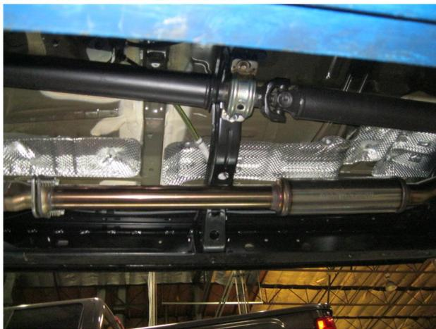
**Step 3.** Begin installation of your new MAGNAFLOW system by attaching the Inlet Pipe Assembly to the catalytic converter outlet using the OEM fasteners and insulator. Keep all fasteners and clamps loose until final adjustment.
