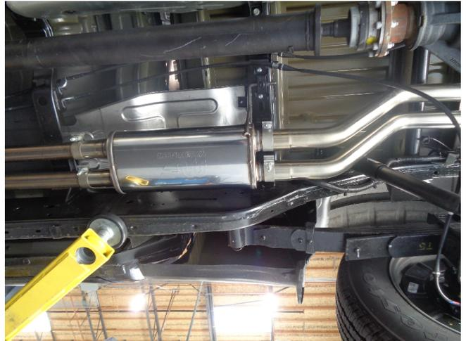
Step 4: Loosely attach the Muffler Assembly to the Extension Pipes using the supplied 2.25" clamps and engaging the welded hanger into the rubber insulator. Next install the Over Axle Pipes to the outlets of the Muffler Assembly using the supplied 2.50" clamps. (These pipes are identical).
