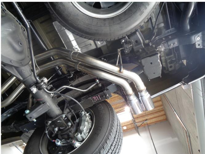
Step 5: Finish by installing the Tailpipe Assembly to the Over Axle pipes using the supplied 2.50" clamps and fitting the hanger into the rubber insulator.
