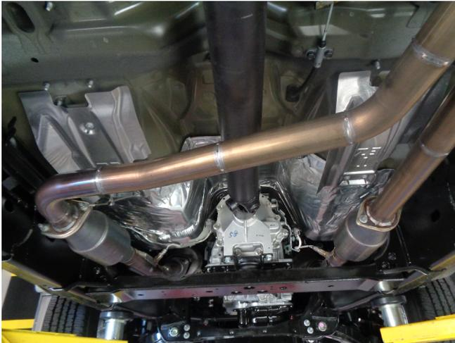
Step 2: Begin installing your new system by loosely bolting both inlet flanges of the D/S and P/S Inlet Pipe Assemblies to the catalytic converter outlets using the OEM hardware. Engage the D/S hanger to the rubber insulator.
