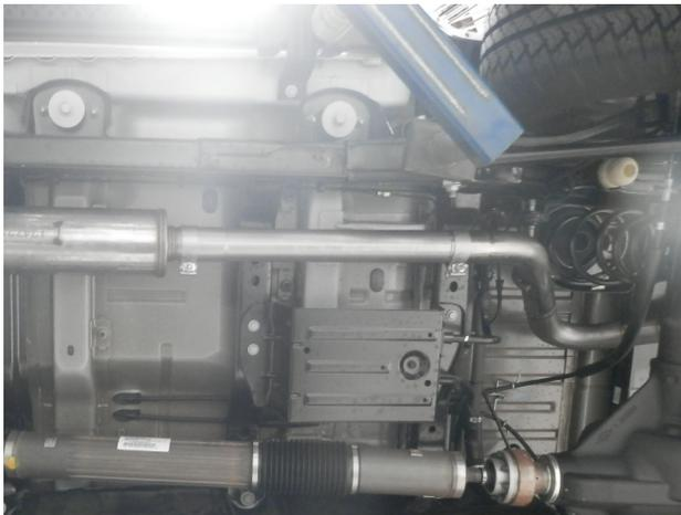
Step 4: The included Extension Pipe is required for the four door model only. It is to be installed between the Resonator Assembly and the Over-Axle Pipe. If you have the two door model this pipe may be discarded.
