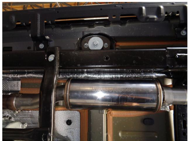
Step 3: Begin installation of your new MAGNAFLOW system by attaching the Resonator Assembly to the catalytic converter outlet using the OEM clamp. Engage the welded hanger to the rubber insulators. Keep all fasteners and clamps loose until final adjustment.
