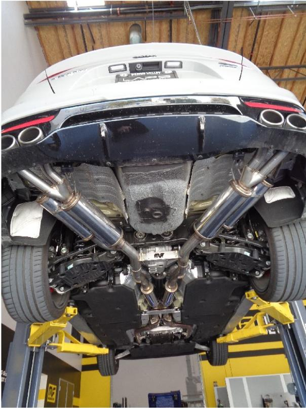
**Step 4:** Once a final position has been chosen for the new exhaust system, evenly tighten all clamps from front to rear using the torque specifications on page one of these instructions. Tighten fasteners for Muffler brace and install factory underbody brace. Inspect all fasteners after 25-50 miles for operation and re-tighten if necessary.
