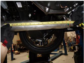
**Step 1.** It is necessary to cut the factory exhaust system to install the new Magnaflow unit. To do this measure rearward from the welded hanger forward of the rear muffler. Measure and cut 16" for the drivers side and 17" for the passengers side as shown. Deburr the cut pipes to facilitate installation of the new system.
