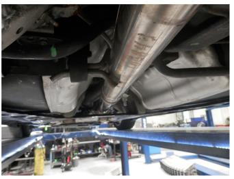
**Step 4.** Next loosely attach the Mid Pipe Assembly to the Inlet Pipe Assembly using the supplied clamp. Engage the welded hanger to the rubber insulator.
