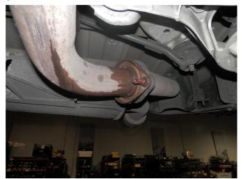
**Step 2.** Unbolt the flange junction between the mid pipe and the muffler assembly. Disengage hangers from rubber insulators and remove the OEM exhaust.
