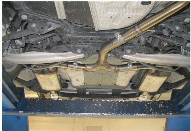
**Step 3.** Next Install the Extension Pipe Assembly to the outlet of the Resonator Assembly using the supplied 2.50" clamp. Then install the Y-Pipe Assembly to the Extension Pipe Assembly in the similar fashion using the supplied 2.50" clamp, and fitting the welded hangers into the rubber insulators.
