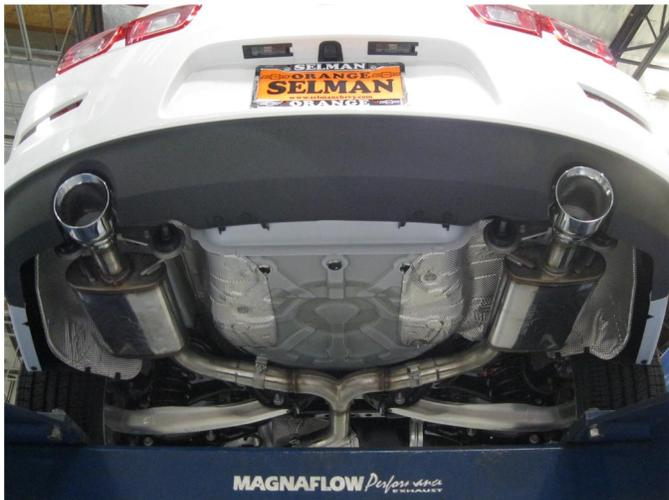
**Step 4.** Finish by installing the Muffler Assemblies to the Y-Pipe Assembly using the supplied 2.50" clamp, and fitting the welded hanger into rubber insulator.
