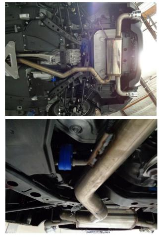
**Step 3.** Next attach the Mid Pipe Assembly to the Inlet Pipe using a supplied 2.50" clamp. Insert the hanger into the rubber insulator. Finish by attaching the Muffler Assembly to the Mid Pipe using a supplied 2.50" clamp and inserting the hangers into the rubber insulators.
