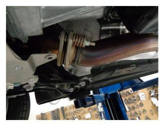
**Step 2.** Begin installation of the new system by fastening the Inlet Assembly to the outlet of the OE exhaust using the spring bolts and the supplied round gasket. leave all clamps and fasteners loose until final adjustment.
