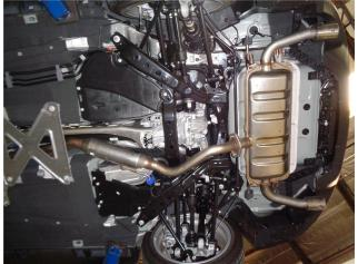
**Step 1.** Begin removal of the exhaust system by removing the underbody cross brace. Next, unfasten the two bolt flange at the front of the exhaust system. With the exhaust system supported, working front to rear extract the welded hangers from the rubber insulators and remove the exhaust as one piece. Retain the flange spring bolts and rubber insulators as they will be re-used on the new Magnaflow exhaust system.
