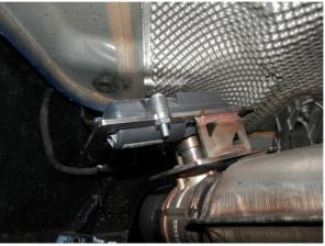
Step 2. Once the OE system is on the ground you will need to swap the servo motors from the factory control valves to the control valves on the Magnaflow Tip Assemblies. Use the new supplied hardware to attach the servo motors the the valves. At this point remove and retain the OE slip clamps to use on the new system.
