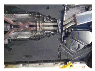
Step 4. Next attach the Resonator Assembly to the X-Pipe Assembly using the OEM clamps and fitting the hangers into the rubber insulators
