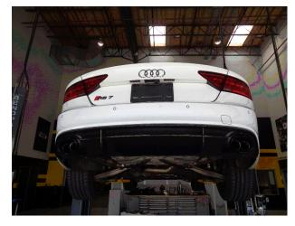
Step 7: Once a final position has been chosen for the new exhaust system, evenly tihgten all clamps from front to rear using the torque specifications on page one of these instructions. Inspect all fasteners after 25-50 miles for operation and re-tighten if necessary.
