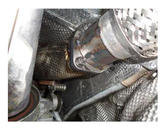
Step 3. Begin installation of the new system by fastening the X-Pipe Assembly inlets to the catalytic converter outlets using the OE fasteners (Leave all clamps and fasteners loose for final adjustment of the complete system.)
