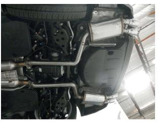
**Step 2.** Begin installation of the new system by fastening the inlet flanges of each Muffler Assembly to the outlet flanges of the catalytic converters using the OEM spring and bolt along with the supplied gaskets and hardware. Locate the each welded hanger into the OEM rubber insulator.
