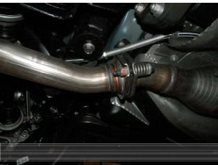
**Step 1.** To remove the OEM exhaust system you will first need to remove the four spring loaded bolts at the flange junction that attach the OEM muffler assemblies to the vehicles catalytic converters. Disengage all welded hangers from the rubber insulators. Be careful not to damage any mounting hardware as it will be needed to install your new system.
