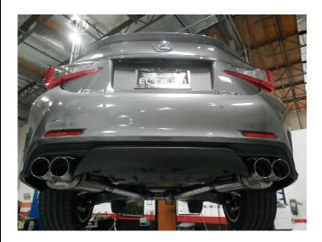
**Step 3.** Once a final position has been chosen for the new 6system, evenly tighten all clamps from front to rear using the torque specifications on page one of the instructions. Inspect all fasteners after 25-50 miles of operation and re-tighten if necessary.
