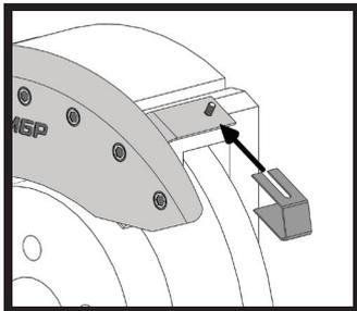
Slide the stainless steel clips over the bridges and caliper brackets and around the threaded studs to fasten the cover. Fit should be snug and secure.
