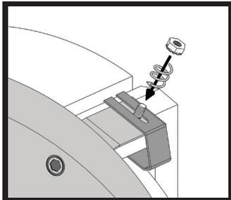
Install the supplied locknuts onto the threaded studs to secure clip to bridge. Tighten with 3/8-inch wrench or socket to 25 inch - pounds (about 1/4 turn past finger-tight). Do not over tighten.
