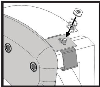
Install the supplied locknuts onto the threaded studs to secure bridge to clip. Tighten with 3/8-inch wrench or socket to 25 inch-pounds (about 1/4 turn past finger-tight). Do not over tighten.
