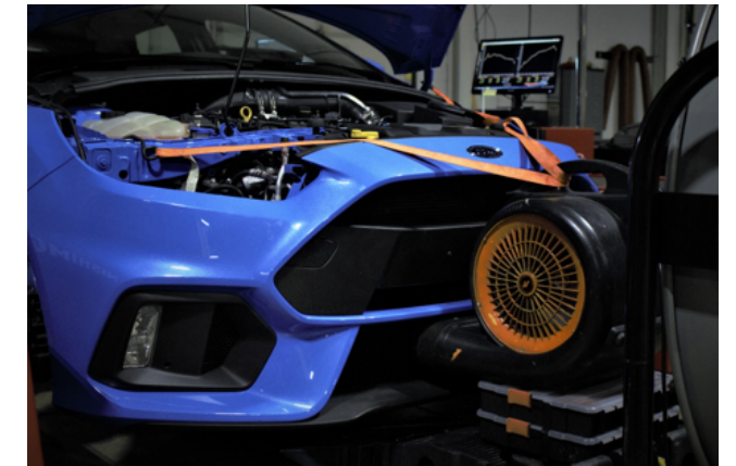
FIGURE 10: A Dynapack dynamometer was used for vehicle testing.
