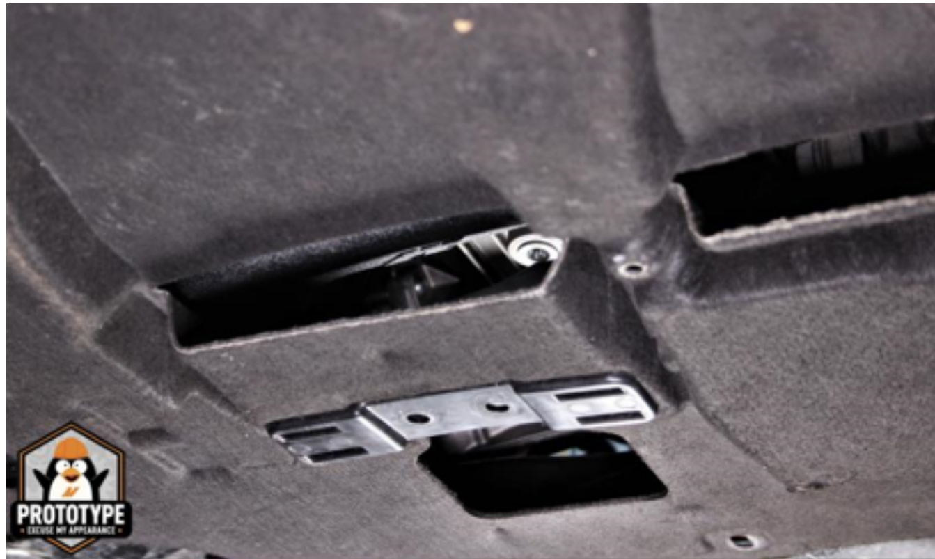
FIGURE 8: Image of the Mishimoto hot-side intercooler pipe installed with the lower splash shield in place showing that it does not obstruct air flow to the heat sink on the bottom of the PTU.
