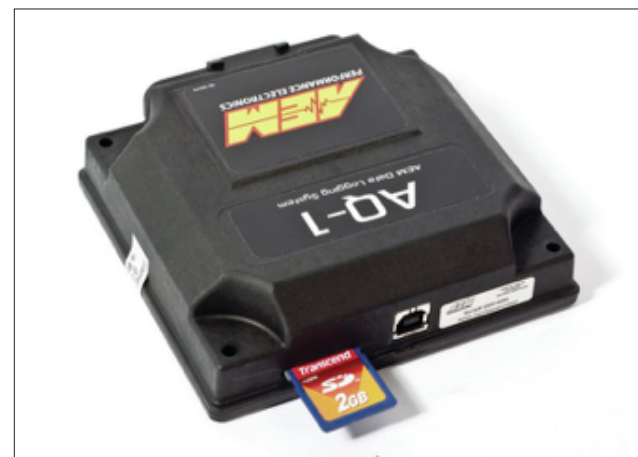
FIGURE 9: AEM AQ-1 Data Logging System
