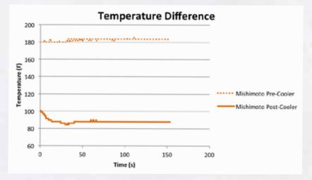
The efficiency is very high for this test vehicle under the conditions stated above. Depending on the vehicle type, driving conditions, and weather conditions, results may vary. Pressure loss averaged 2.5 psi for the Mishimoto 25-row oil cooler. No harm to the engine will occur by adding this cooler to your system.
