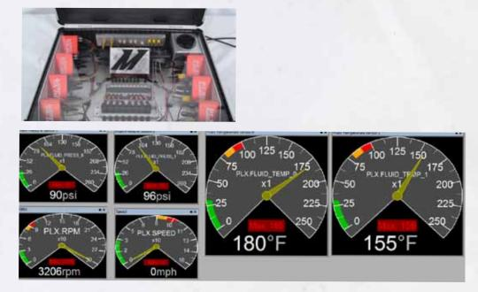
Fluid temperatures were taken from both the inlet and outlet of the 25-row oil cooler, using custom inline sensor housings and PLX fluid temperature sensors. Oil pressure was also tested to ensure that no dramatic pressure drop occurs when installing the oil cooler.
