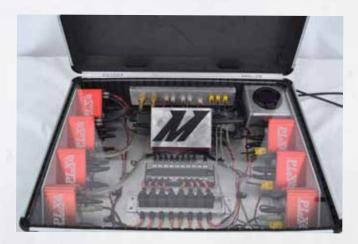
Fluid temperatures were taken with PLX fluid temperature sensors from both the inlet and outlet of the standard Mishimoto oil sandwich plate. Oil pressure was also measured to ensure that no dramatic pressure drop occurs when installing the oil cooler.
