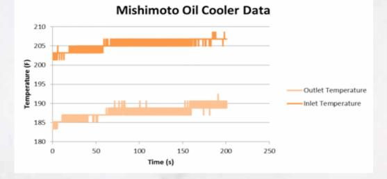
At cruising speeds, the oil temperatures entering the cooler are around 203-207 degrees F. The graph above shows that, under cruising conditions, the Mishimoto oil cooler reduced temperatures by approximately 20 degrees on average.
