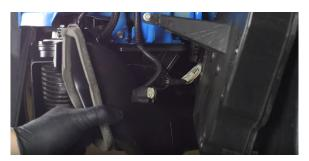
12. Loosen the clamp securing the hot-side pipe to the intercooler end tank. Then, separate the connection. (1x worm gear clamp)
