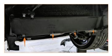
> Measure and mark right side of the air duct.
