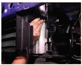
21. Reinstall the intercooler and secure it with the two 8mm bolts. [2x 8mm bolts]
