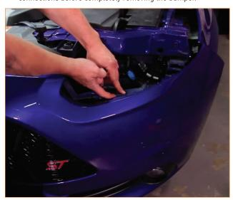
12. Remove the upper air shroud by releasing the two clips at the outside edges.
