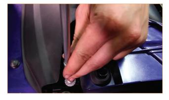
04. Remove the four pop-clips along the top of the bumper cover located in the engine bay. (4x pop-clips)
