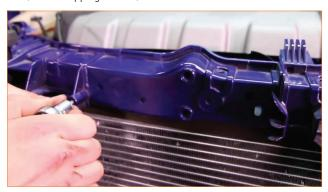
26. Install the lower mounting bracket onto the oil cooler using the supplied 10mm nuts and bolts. This bracket installs on the passenger side of the oil cooler and attaches it to the crash beam. (3x 10mm nuts, 3x 10mm bolts)
