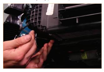
20. Remove the active grille shutters. The shutters are held in by four clips that secure it to the AC condenser. These can be released by hand. Then slide the active grille shutters down and remove them completely. They will not be reinstalled.
