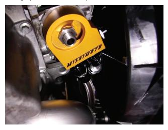
31. Locate the longer oil cooler line in your kit. Route this line along the top of the intercooler, and attach the 90-degree fitting to the passenger-side fitting on the oil cooler, but do not fully tighten. Loop the line directly around the radiator on the driver side.
