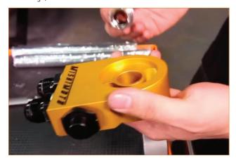
29. Lubricate the rubber seal on the sandwich plate using clean motor oil, and wipe off the mating surface on the engine where the oil filter was removed.
