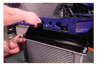
25. Locate the two unthreaded holes along the upper edge of the radiator support. The oil cooler mounting bracket will align with these holes. Carefully tap these holes with the provided self-tapping screws. Run the screws in by themselves to create threads. Make sure the self-tapping screws are driven in straight to avoid damaging the radiator support. Then remove the self-tapping screws and install the oil cooler and bracket. (2x self-tapping screws)
