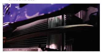
32. Locate the shorter oil cooler line in your kit. Route this line next to the first line, and attach the 90-degree fitting to the driver-side fitting on the oil cooler, but do not fully tighten. Loop the line directly around the radiator on the driver side.
