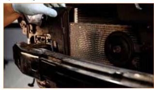
**4.** Bolt the oil cooler bracket to the support beam using the two supplied 10mm bolts.
