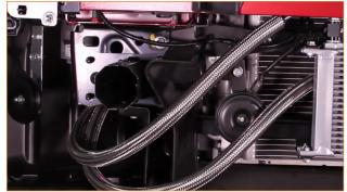
**28.** Fully tighten both oil line fittings onto the oil cooler.
