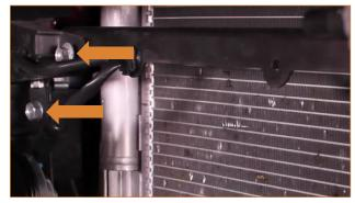
14. Install the three provided brackets to the oil cooler. To orient the cooler, the fittings are at the top, and the Mishimoto M logo will face forward. The longest bracket attaches to the bottom of the oil cooler on the passenger side. The shortest bracket attaches to the top of the cooler on the driver side. The remaining bracket attaches to the top of the cooler on the passenger side. [6x 10mm bolts, 6x nylon-insert lock nuts]
