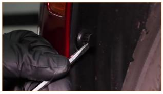
05. Gently pull back the fender liner to expose a Phillips screw that attaches the bumper cover to the fender. Remove this screw on both sides. (2x Phillips screws)
