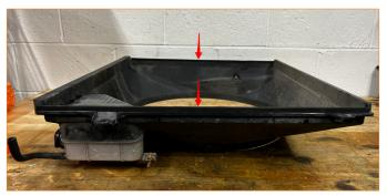
03. For 2005-2015 models, install the Mishimoto radiator the same way you would install a stock radiator. Secure the fan shroud to the radiator with provided hardware.
