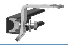
2. Install mounting brackets into the cargo rails. Assemble the brackets as shown and insert into the cargo rail. Three brackets per side are required. Note: You may reinstall tie downs at this time in between mounting brackets.
