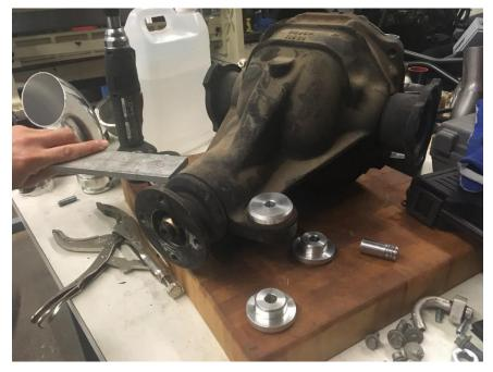
**Step 6:** Now begin to press or hammer the subframe differential bushings in, ensure the flat side is facing the front of the vehicle.
