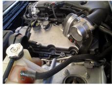
2 Remove nut securing OEM air box, save for later steps . Disconnect rubber PCV hose from side of air box.
