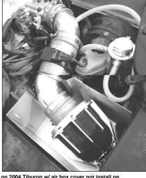
Install the SW dual pipe on the throttle body side. Dragon Intake install on 2004 Tiburon w/ air box cover not install on If you have any quesiton about this product, Please refer to our website @WWW.WEAPON-R.COM
